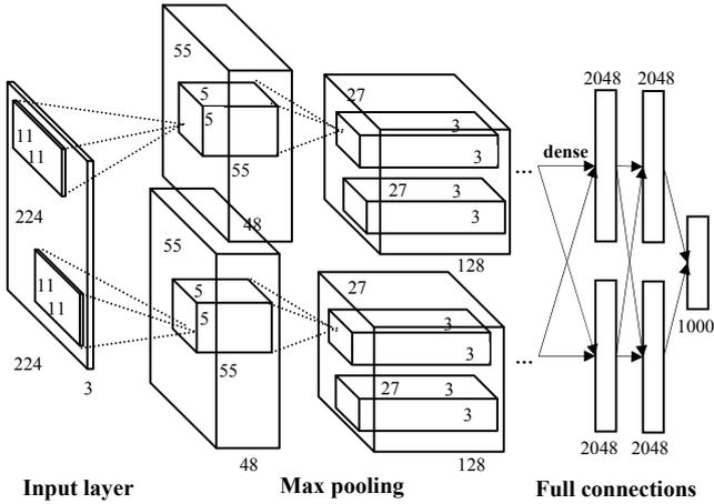
**Figure 5. The deep architecture adopted in DCNN for ImageNet classification.**
